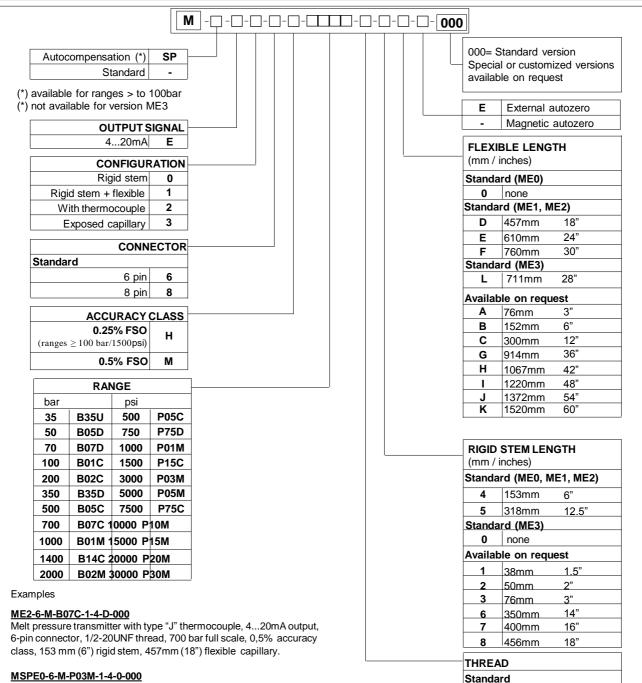
Melt pressure transmitter autocompensated version, rigid stem, 4...20mA output, 6-pin connector, 1/2-20UNF thread, 3000 psi full scale, 0,5% accuracy class, 153 mm (6") rigid stem.
